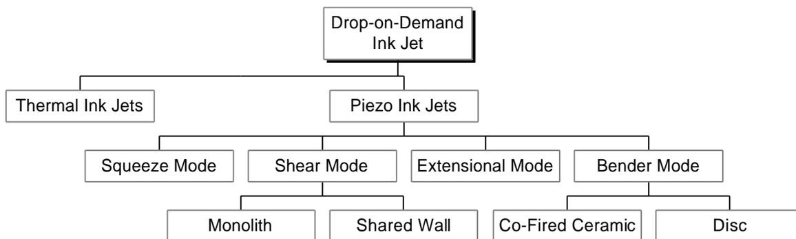
Figure 1. Schematic of various types of Drop-on-Demand Ink Jets.
