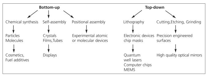
Figure 4.1 The use of bottom-up and top-down techniques in manufacturing
