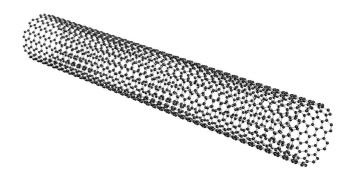
Figure 3.1b Schematic of a multi-walled carbon nanotube (MWNT)
