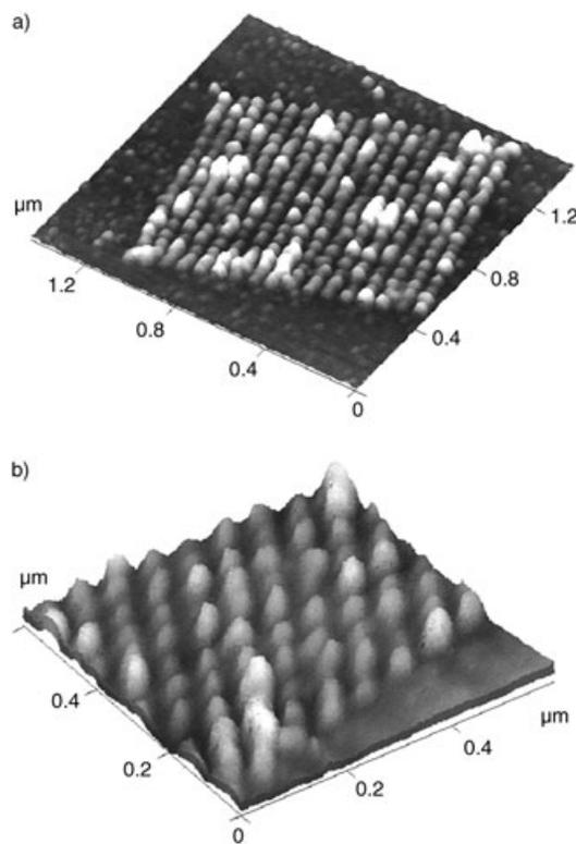
**Figure 3.** Uniformly covered array of individual iron particles with a next-neighbor spacing of  $\approx 50 \text{ nm}$ . Imaging is performed in tapping mode with a Multimode SFM.
