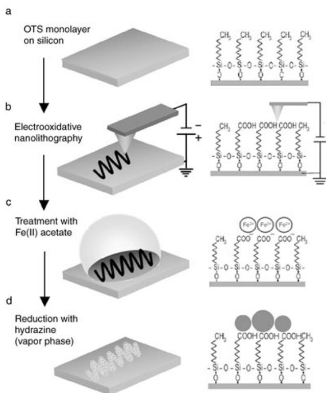
**Scheme 1.** Schematic representation of the fabrication approach of magnetic nanostructures on OTS self-assembled monolayers (a) by means of electrooxidative nanolithography (b) followed by the site-selective in situ derivatization of the surface structures (c, d).
