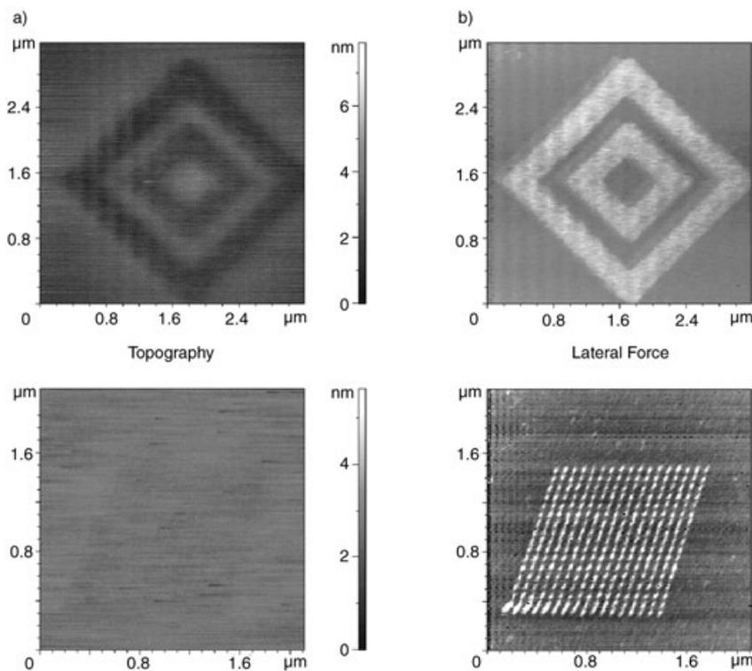
**Figure 1.** a) Topography and b) lateral force microscopy images of the OTS self-assembled monolayer after the electrooxidative template inscription. The bright lateral force contrast and the almost unaffected topography contrast are regarded as an indication of the successful conversion of surface-terminated  $-\text{CH}_3$  groups into  $-\text{COOH}$  functions.
