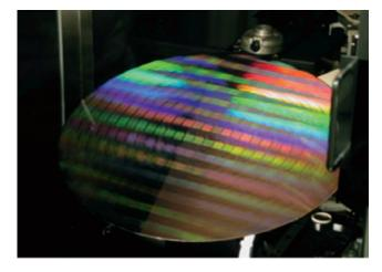
**Figure 2.** An optical modulator made entirely out of a silicon wafer.<sup>[79]</sup> The evolutionary extension of the technology for micrometer-scale fabrication into the sub-100-nm range guarantees that "nanotechnology" will happen.
