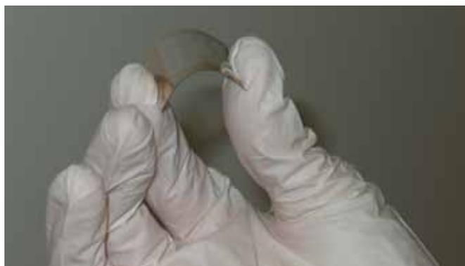
Fig. 6 Photo of an RFID tag component circuit. (Courtesy of OrganicID Corporation.)
