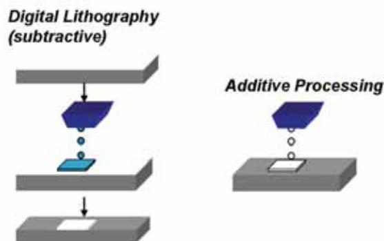
Fig. 7 Illustrations of additive and subtractive (digital lithography) jet-printing processes. (Reprinted with permission from<sup>4</sup>. © 2005 Korean Information Display Society.)
