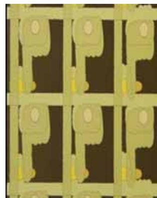
Fig. 8 Photograph of an array of amorphous Si TFTs patterned using digital lithography. The pixel size is  $340\ \mu\text{m}$ .
