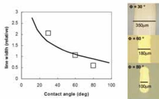
Fig. 4 Calculated line width as a function of wetting contact angle, assuming a small cylindrical liquid pattern. Data points and photographs show line width measurements for a Ag nanoparticle ink printed on surfaces of different contact angles.
