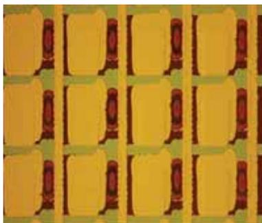
Fig. 11 Photograph of a TFT array fabricated at PARC with jet-printed PQT12 polymer. The other layers are patterned using digital lithography. The backplane is designed for a reflective display.
