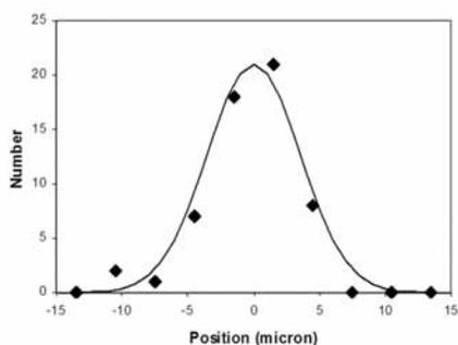
Fig. 3 Histogram of jet-printed drop position deviation in the print direction  $\Delta x$  for  $\sim 50$  drops from individual ejectors in a multiejector print head compared with a Gaussian distribution having a standard deviation of  $3.5 \mu\text{m}$ . The print head has velocity normalization.
