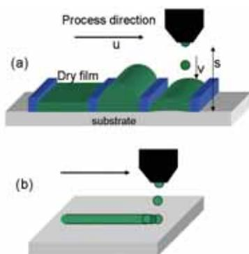
Fig. 6 Schematic showing (a) printing into a previously fabricated well, as used for PLEDs and color filters, and (b) printing unconstrained lines on a free surface. The head velocity  $u$ , the drop velocity  $v$ , and the head-substrate gap  $s$  are indicated.
