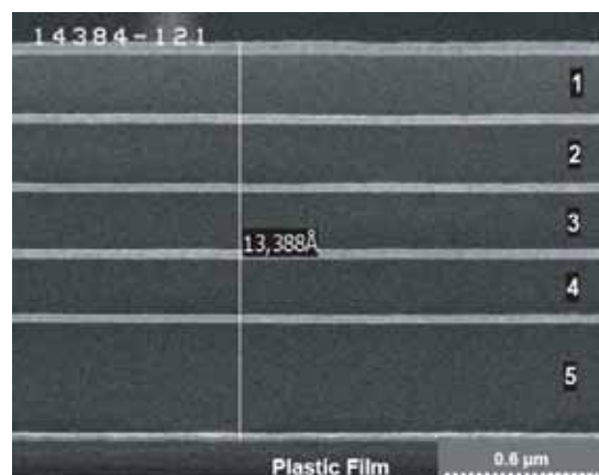
Fig. 3 Organic/inorganic multilayer structure from Vitex Systems. (Reproduced courtesy of Vitex Systems.)
