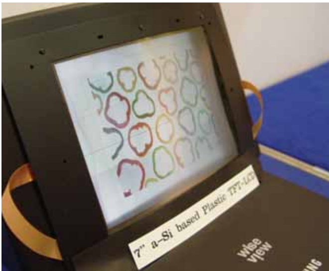
Fig. 4 Full-color TFT-LCD on PES by Samsung Electronics.
